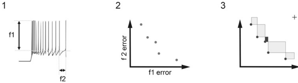
Fig. 10.3 Illustration of central concepts for reconstructing biophysical neuron models. (1) Features are extracted from electrophysiological recordings. (2) Pareto set of solutions plotted for two dimensions (two objectives) of a
