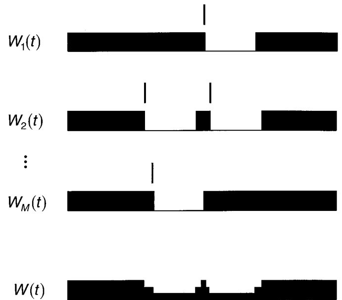
Figure 3. Schematic illustration of the derivation of W(t) , the probability of free firing. On each trial j , W_j(t) (solid gray) has a value of zero during the refractory period following a spike (vertical lines) and one elsewhere. This function is averaged over all trials (bottom), to yield W(t) , the fraction of trials during which free firing was possible at time t .
